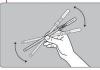
In the lab, vigorously shake or vortex the swab for 10 seconds, to release bacteria from the swab tip.
