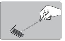
Hold the swab handle to make a 30° angle 5 with the surface. Rub the swab slowly and thoroughly over the desired surface area. Rub the swab three times over this surface, reversing direction between alternating strokes.
