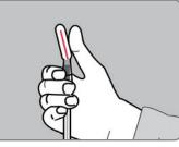
Prepare the swab by holding it with the bulb end near your thumb. Bend the red snap valve, at a 45° angle until you hear the valve break. This allows the letheen broth to flow into the tube end and wet the swab.
