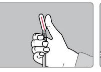
At the sampling location, prepare the swab by holding it with the bulb end near your thumb. Bend the red snap valve at a 45° angle until you hear the valve break. This allows the letheen broth to flow into the tube end and wet the swab.
