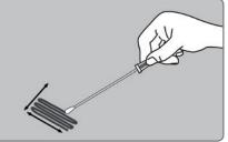
Hold the swab handle to make a 30° angle with the surface. Rub the swab slowly and thoroughly over desired surface area. Rub the swab three times over this surface, reversing direction between alternating strokes.
