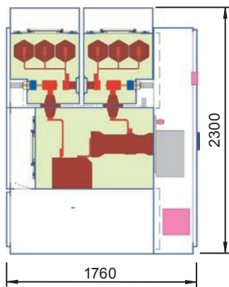
Fig. 7.1.2.1.1: Sectionaliser panel 1250 A with block-type CT or sensor
