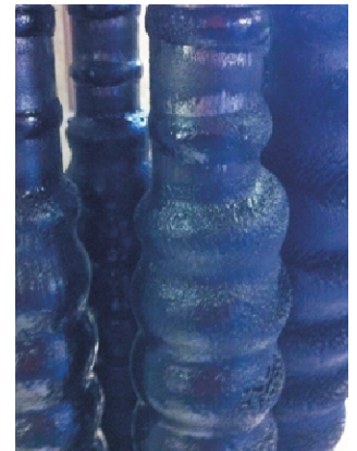
Ferritic particles on magnetic filter rods
