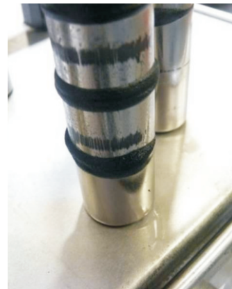
Finest debris collected on magnetic filter rod
