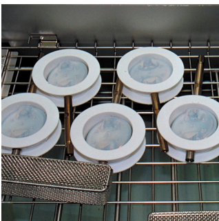
Cleansing the parts with ultrapure water
