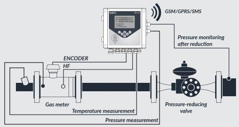
4. Process of measurement using MacBAT 5 (with external pressure sensor) and rotary gas meter
