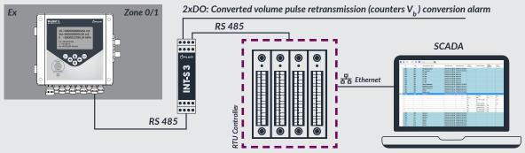
3. Process of measurement using MacBAT 5 and turbine gas meter
