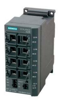
SCALANCE X208, MANAGED IE SWITCH, 8 X 10/100MBIT/S RJ45 PORTS, LED DIAGNOSTICS, ERROR SIGNAL CONTACT WITH SET BUTTON, REDUNDANT POWER SUPPLY, PROFINET-IO DEVICE, NETWORK MANAGEMENT, INTEGRATED REDUNDANCY MANAGER, INCL. ELECTRONIC MANUAL ON CD, C-PLUG OPTIONAL
