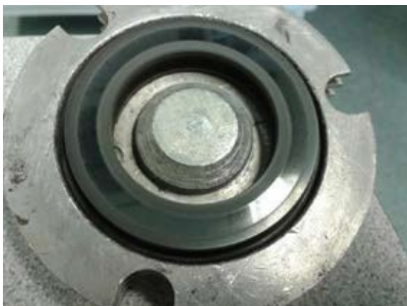
CVD diamond coated sealing surface, as seen after 10 hours of dry running at 1500 rpm.
